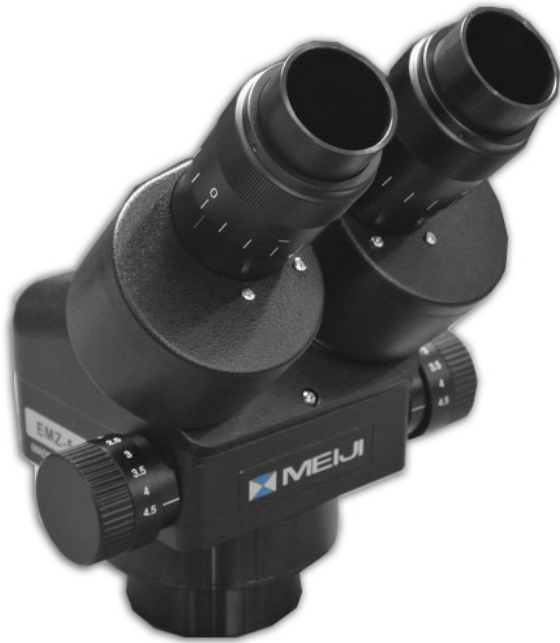
EMZ-5/BLACK (0.7X–4.5X) Binocular Greenough Design, Stereo Zoom Body, Working Distance 3.7" (93mm)
