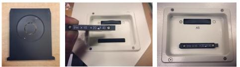
Note: To adjust iris, move the top iris wheel (AS) to desired position
