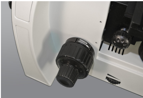
Coaxial Coarse and Fine focus Knobs
