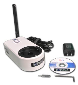
HD-UWF: Integrated Wifi, USB 2.0 Camera for Meiji Techno MT Series with dovetail mount for MT series software. Connects via WIFI or USB 2.0 to PC/laptop. Not MAC compatible.
